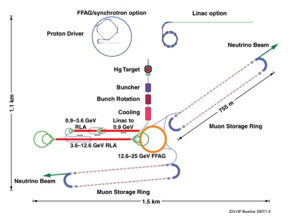
Figure 1: Schematic drawing of the ISS baseline 2007/1.0 for the Neutrino Factory accelerator complex [1]. The various systems have been drawn to scale.
